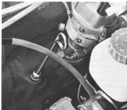
2 Checking the oil level in the engine
